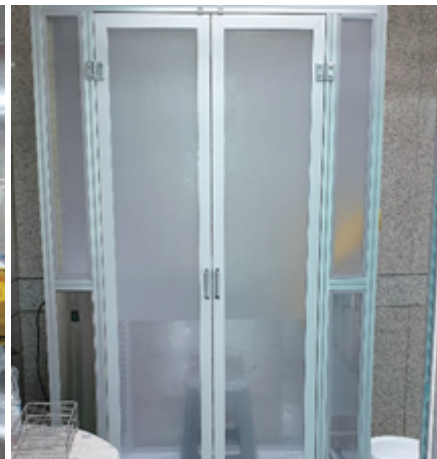
Glovebox negative pressure booth (subject view, side)
